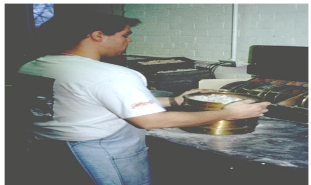
8) A gradation test is performed
