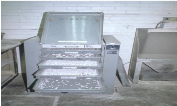
3) Sample is sieved into individual fractions
