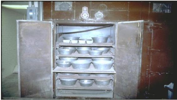
2) Sample is dried to a constant weight
