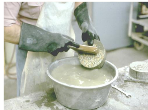
Preparing a sample for the circular track
