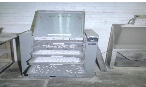
3) Sample is sieved into individual fractions
