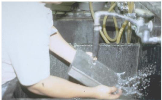
6) Sample is rinsed of the solution & dried
