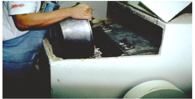
6) Material is placed in the LA Abrasion machine
