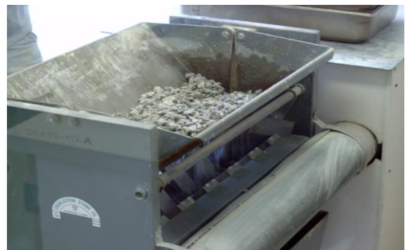
A coarse aggregate mechanical splitter for reducing aggregates to sample size
