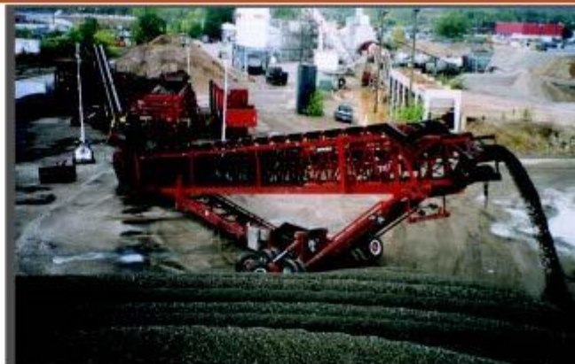
WINDROW STOCKPILING WITH A TELESCOPING CONVEYOR F21
