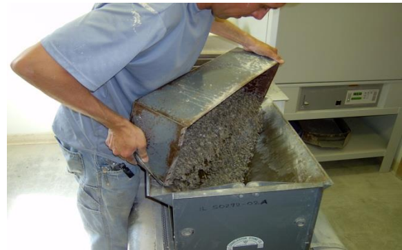
The material is reduced to test sample size
