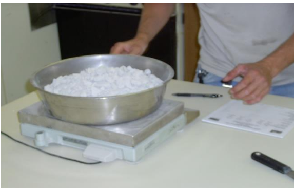
4) Material is weighed based on size
