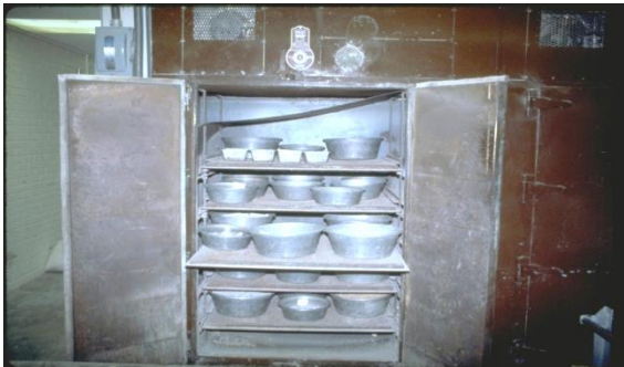
2) Sample is dried to a constant weight
