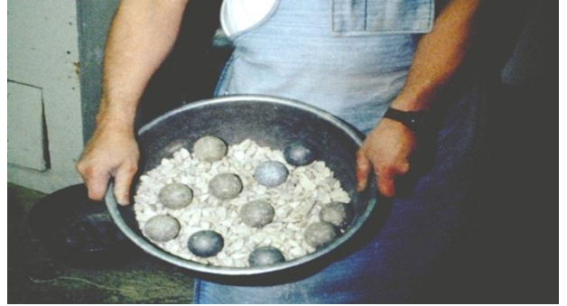
5) Steel balls are added based on quality
