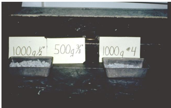
4) Sample size is based on the gradation
